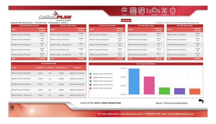
A Dashboard report consists of data corresponding the top sensor events (major or micro), top valve events (major or micro), top robot events and top safety events. Faults that are generated are updated under the "Live Downtime Events" section. Each fault can be clicked on for more in-depth details.
