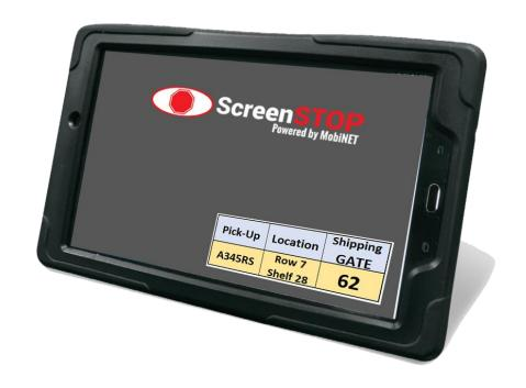
ScreenSTOP is a patent-pending intelligent in-motion technology solution used for instant screen masking for vehicles in motion, eliminating the hazards associated with in-vehicle computer displays installed on lift trucks and other vehicles.
